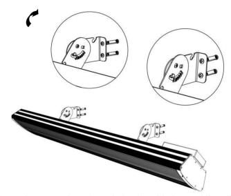
7. Securely engage them through the slotted holes, enabling slight rotational adjustments of the product to different positions.
