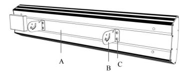
6. Interlock the hanging tabs on the two articulating brackets (B) attached to device (A) with the hanging tabs on the corresponding two brackets (B) on the wall. Pass them through the slotted holes and secure them firmly. Afterward, gently shake the unit to ensure there is no detachment.
