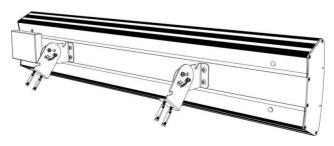
8. Insert the flange nut kits(F) through the pivot hole, securing it with a nut. Next, pass the flange nut kits(G) through the U-shaped groove, adjust it to the desired angle, and secure it by tightening the nut.
