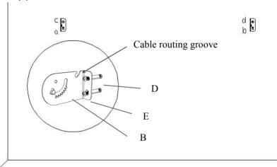
*Note: The cable routing groove on the brackets(B) should face upward.*
