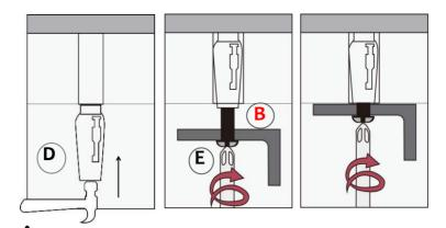
The expanding nut goes into the inside of the hole, it is strictly prohibited to install it in reverse!
